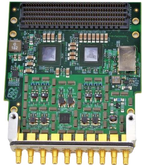
Figure 2: FMC249 Top View without Heatsink
