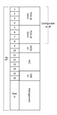
Figure 4: Pinout Block Diagram
