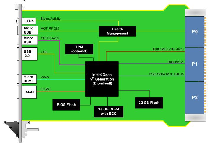
Figure 2: VPX754 Functional Block Diagram
