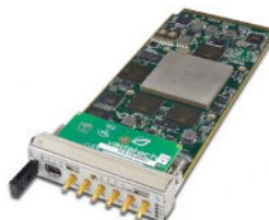
AMC526 AMC Dual ADC, Virtex-7, 12-Bit @ 2.6 GSPS
