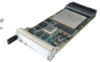
The AMC596 provides an XCVU440, the largest of the Virtex UltraScale™ FPGAs, 8GB of 64-bit wide DDR4, and a P2040 co-processor. Twenty of the GTH transceivers are routed to the tongue 2 PinoutPlus™ connector, allowing the module to make use of the dense connectivity of VT884. This makes the module ideal for constructing dense meshes of closely-coupled FPGAs, capable of addressing complex ASIC and system emulation tasks.
