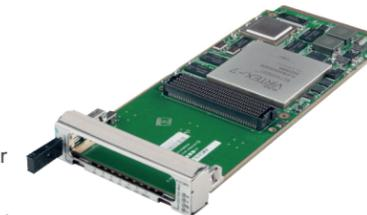
The AMC515 provides an XC7V2000T with P2040 co-processor for local management and up to 2GB of 64-bit wide DDR3. The 200T has almost a million logic cells and over 2,000 DSP slices, supported by GTX (12.5Gb/s) transceivers. It includes a single VITA 57 FMC slot, and offers a lower price/performance point than UltraScale™ modules.
