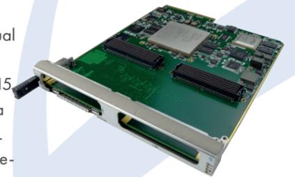
The AMC593 is a dual FMC carrier with an UltraScale™ XCKU115, 8GB of DDR4, and a P2040 co-processor. The board is a double-module size (for the dual FMC slots) so requires a chassis such as VT884 or VT815, and is designed for I/O intensive (edge of emulation network) implementations.
