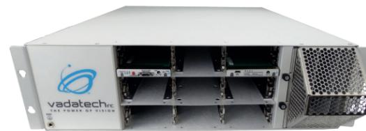
The VT884 can house up to 12 mid-size AMCs, each of which can be up to XCVU440 thanks to the advanced airflow design. Supporting PinoutPlus™, the chassis provides up to 160Gb/s between slots in addition to the standard fabric connections.
