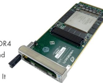
The AMC592 has an UltraScale™ XCKU115 supported by 20GB of DDR4 split over 3 banks (64- and 32-bit wide), giving very high memory bandwidth. It provides a fully-connected VITA 57 FMC slot, making it ideal for implementing external system interfaces at the edge of an emulation network. The KU115 is the largest of the Kintex UltraScale™ FPGAs with over 5,500 DSP slices and GTH (16.3Gb/s) transceivers.
