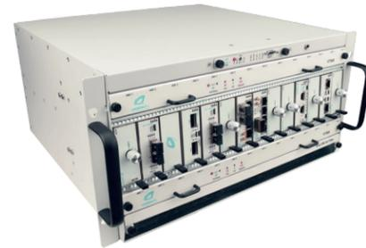
The VT866 provides the power and cooling to support up to 12 full-size AMCs, making it suitable for large, power-hungry FPGAs. The backplane supports 40G links and dual MCH can implement PCIe Gen3, XAUI, SRIO, or low-latency Aurora between the slots.
