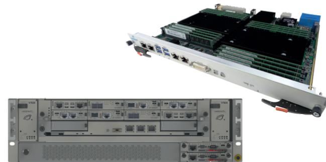
The VT835 provides a 40G backplane and allows a very powerful Intel Blade, such as the ATC126, to be coupled to up to 8 AMC59x AMCs, giving users the ability to mix FPGA and GPP technology in their emulation platform.
