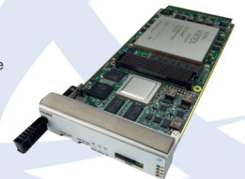
The AMC595 provides an XCVU440, the largest of the Virtex UltraScale™ FPGAs, 8GB of 64-bit wide DDR4, and a P2040 co-processor. The VU440 is well suited to complex ASIC emulation, having 2,880 DSP slices and over 5.5 million logic cells, supported by GTH (16.3Gb/s) transceivers. Note that the FMC slot requires 17.5mm (rather than the more common 10mm) FMC connectors.
