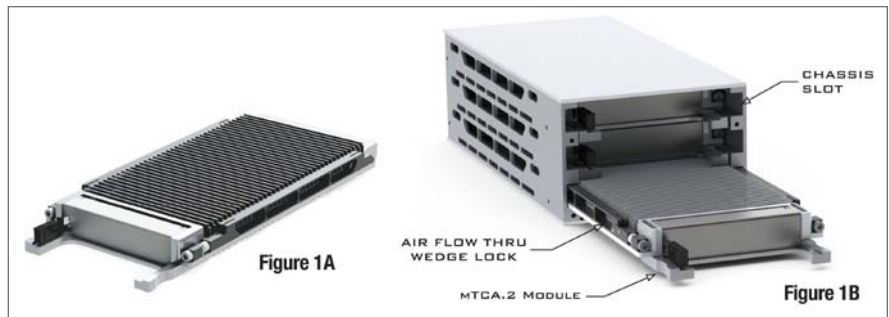
Figure 1 | Pictured are a \mu TCA.2 module (left) and system (right). In a \mu TCA.2 solution, when a module is inserted into the chassis its wedgelocks facilitate thermal dissipation through hybrid air/conduction cooling. Photos courtesy of WaveTherm Corporation in Morrisville, NC.
