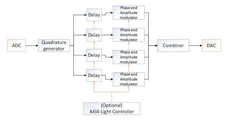
Above we can see that the pulse converted by the ADC is transformed into a complex input and split across a defined number of paths. Each path will be processed with different parameters to represent a different target.
