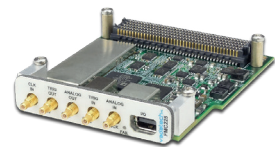
FMC225 ADC, 12-bit @ 4.0 GSPS & DAC, 14-bit @ 5.7 GSPS
