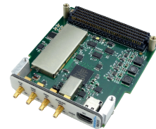
FMC218 FMC High-speed DAC 14-bit at 2.5 GSPS
