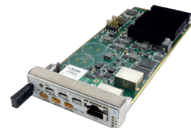
AMC005 AMC Time and Frequency with GPS and IRIG
