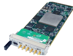
AMC526 AMC Dual ADC, Virtex-7, 12-Bit @ 2.6 GSPS
