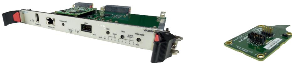
VadaTech VTX980 6U VPX Health Manager w. JSM feature (left) and its JSM to Xilinx or Altera/Intel FPGA JTAG header adapter (right)
