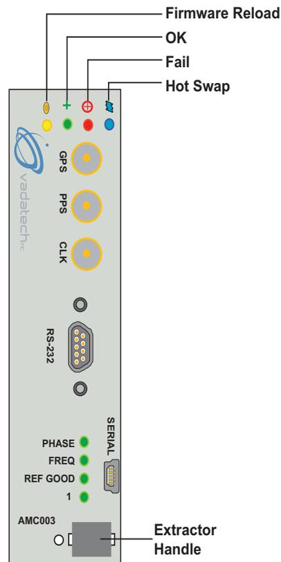
FIGURE 2. AMC003 Front Panel
