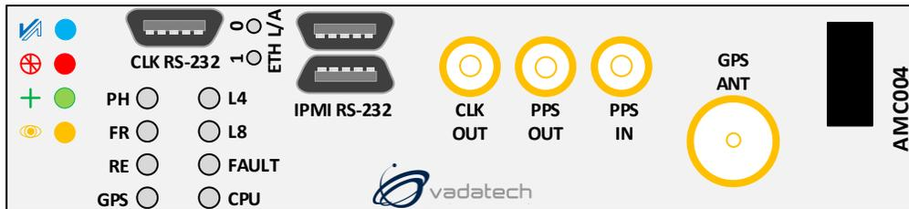
Figure 3: AMC004 Front Panel
