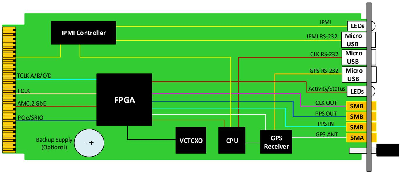
Figure 2: AMC004 Functional Block Diagram
