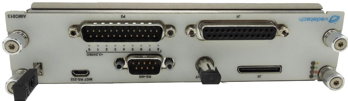
Figure 2: AMC013 Front Panel
