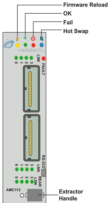
FIGURE 2. AMC113 Front Panel
