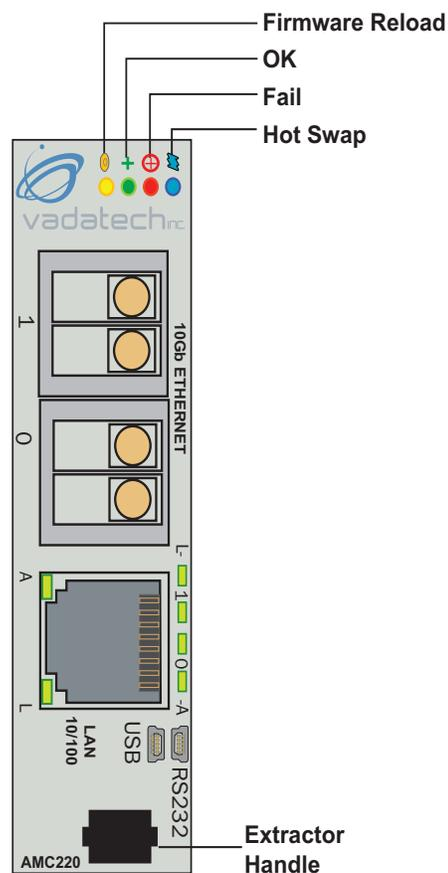
FIGURE 2. AMC220 Front Panel
