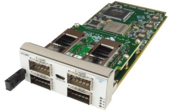
Figure 1: AMC241 with QSFP+
