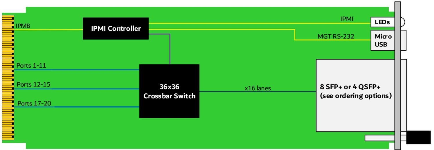
Figure 3: AMC241 Functional Block Diagram
