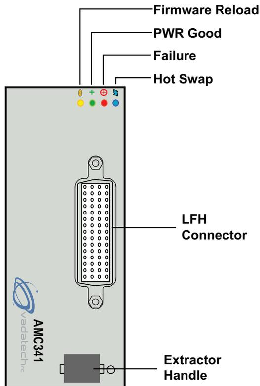
**FIGURE 2.** AMC341 Front Panel
