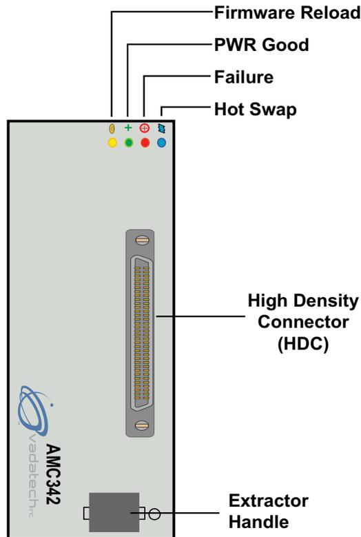
FIGURE 2. AMC342 Front Panel
