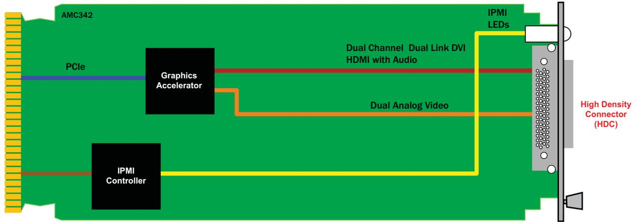
Note: A "Y" adapter cable is needed to take advantage of the dual displays. See ordering options for details.
