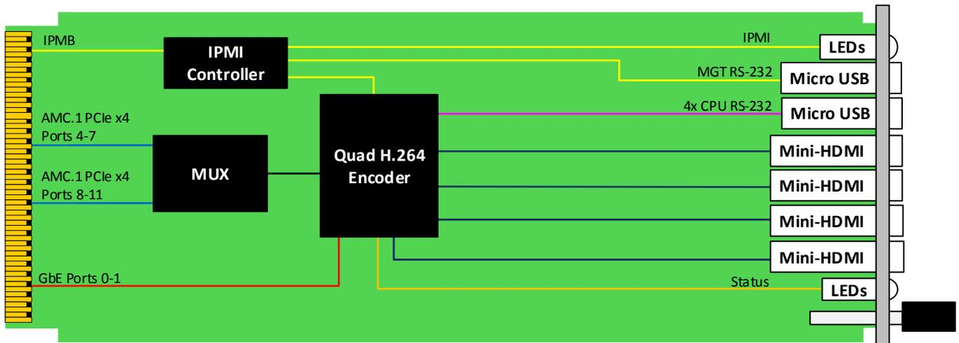
Figure 2: AMC350 Functional Block Diagram
