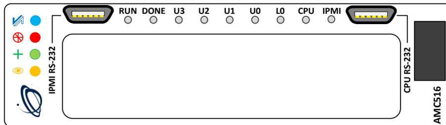
Figure 3: AMC516 Front Panel
