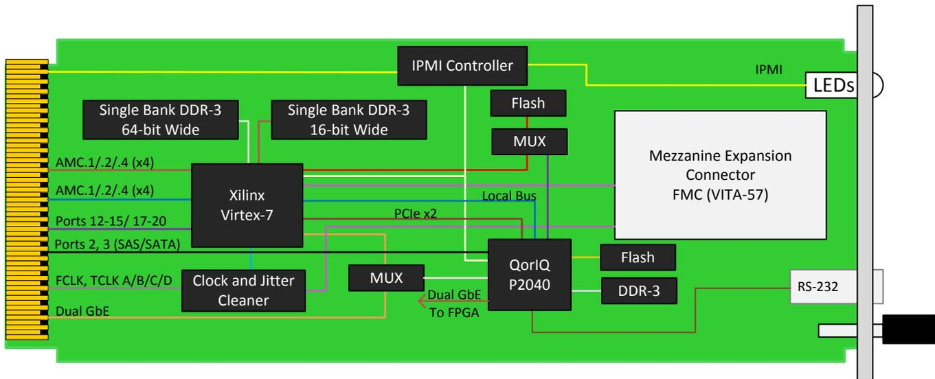
Figure 2: AMC516 Block Diagram
