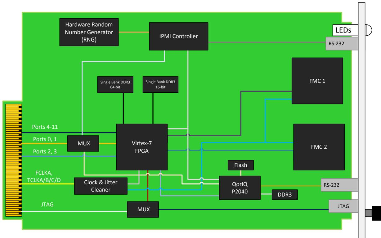
Figure 1: AMC525 Block Diagram
