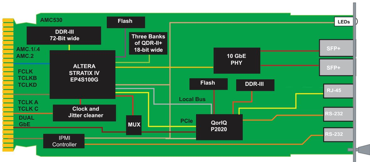
FIGURE 1. AMC530 Functional Block Diagram
