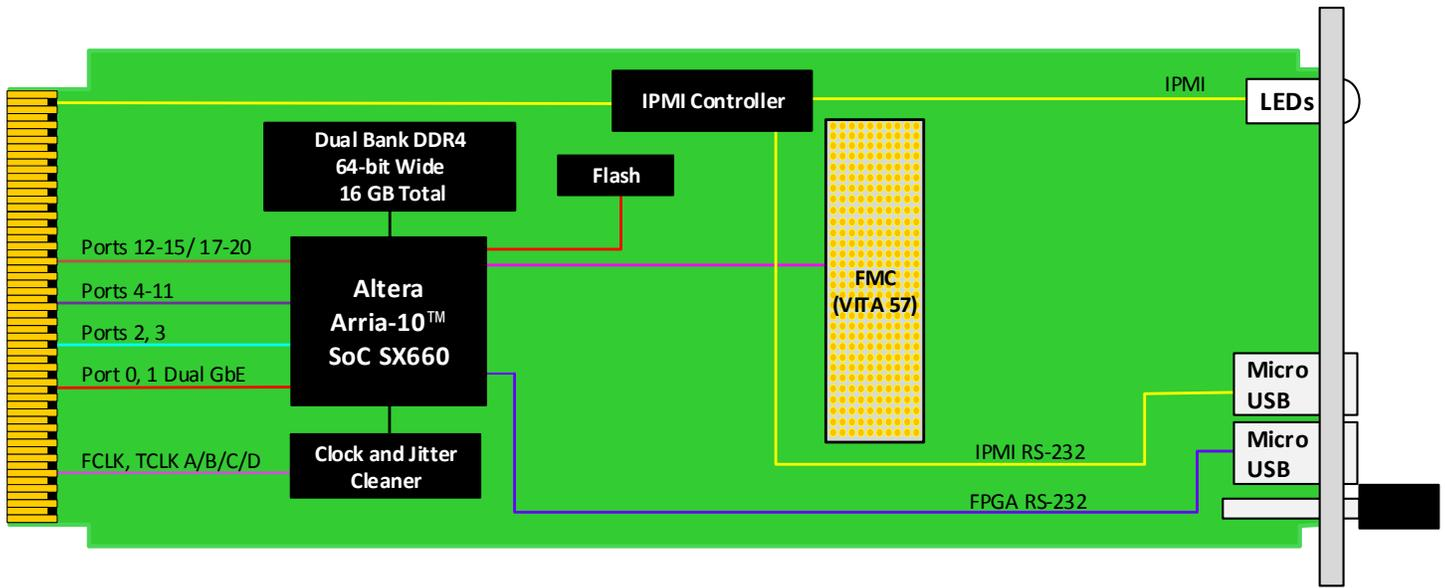
Figure 2: AMC535 Functional Block Diagram
