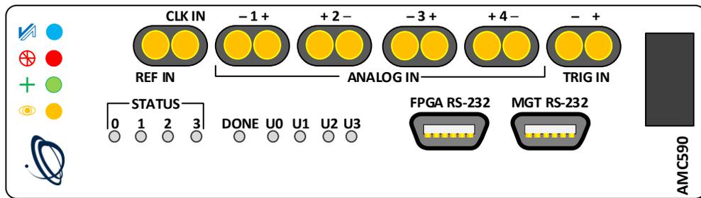
Figure 3: AMC590 Front Panel
