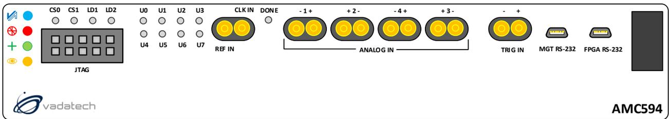
Figure 4: AMC594 Front Panel
