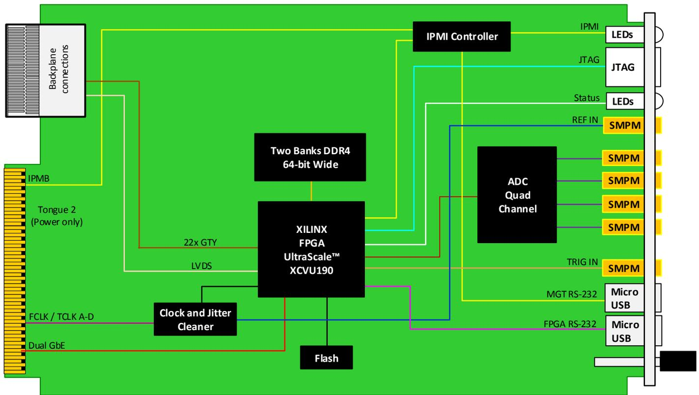
Figure 3: AMC594 Functional Block Diagram
