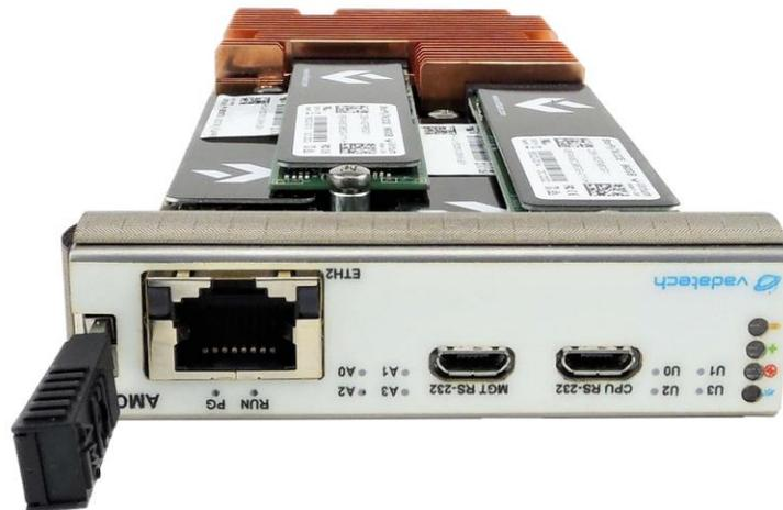
Figure 4: AMC613 Front Panel
