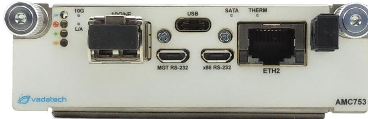
Figure 3: AMC753 Front Panel
