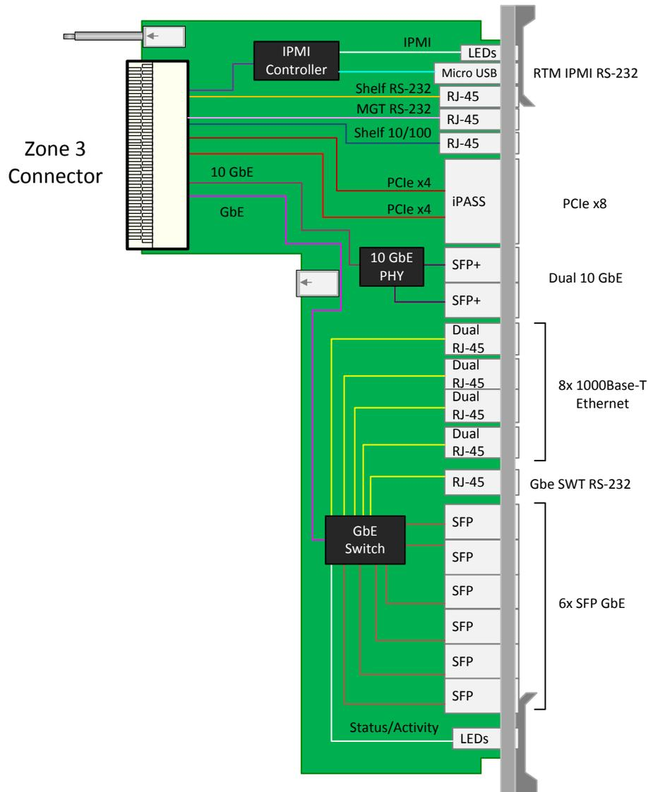
Figure 1: ART001 Functional Block Diagram
