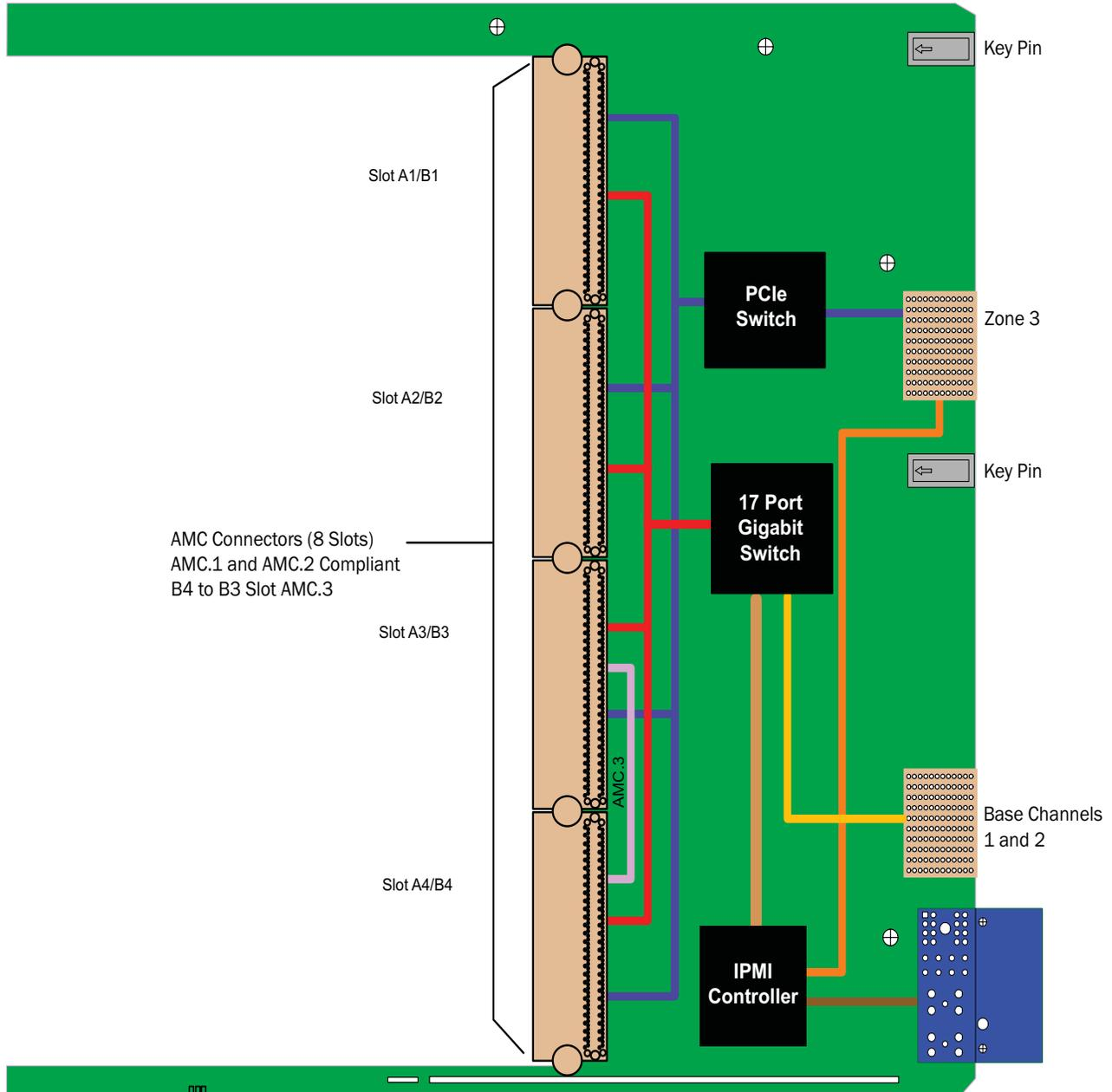
**FIGURE 1.** ATC104 Functional Block Diagram
