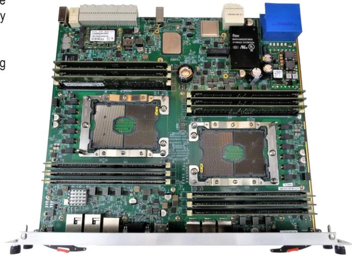
Figure 2: ATC129 Top View Without CPU and Heatsinks
