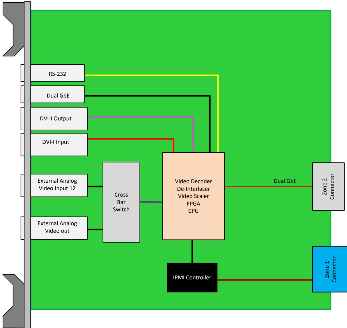
Figure 1: ATC342 Block Diagram
