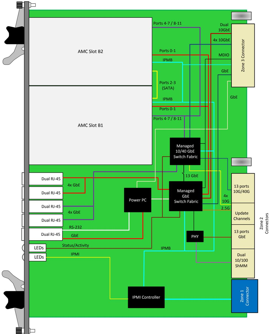
Figure 1: Functional Block Diagram for Option B=0
