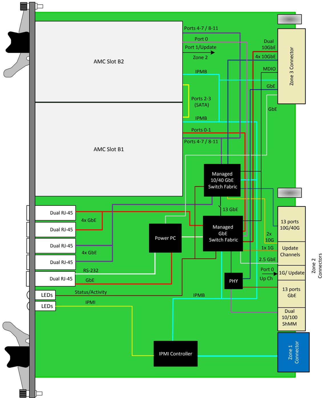
Figure 2: Functional Block Diagram for Option B=1
