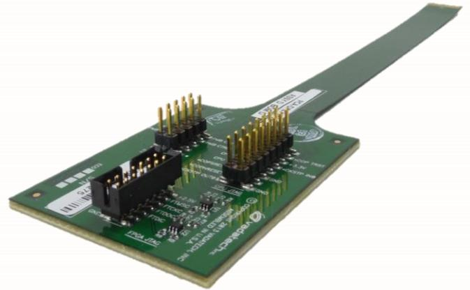
DA234 is a JTAG extender cable that enables standard JTAG pods to be used with VadaTech products fitted with a low profile ZIF connector. The flexible PCB is thin enough to fit between AMC, ATCA and VPX front panels.
