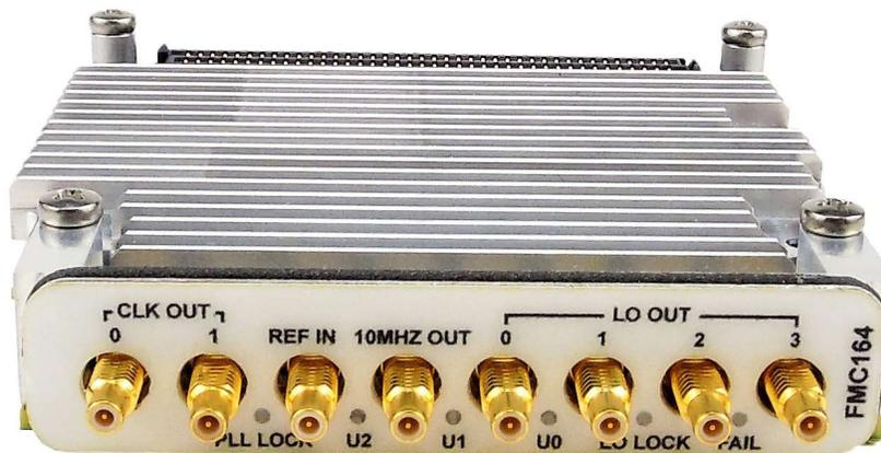
Figure 5: FMC164 Front Panel
