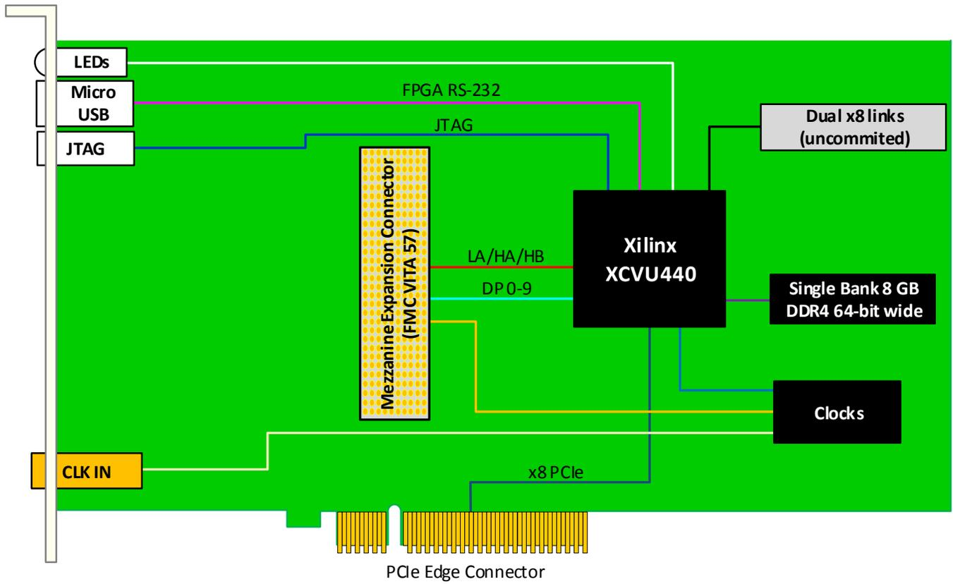
Figure 2: PCI595 Functional Block Diagram
