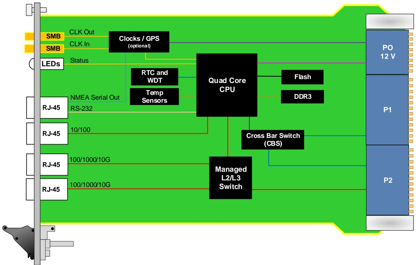
Figure 2: VPX006 Functional Block Diagram
