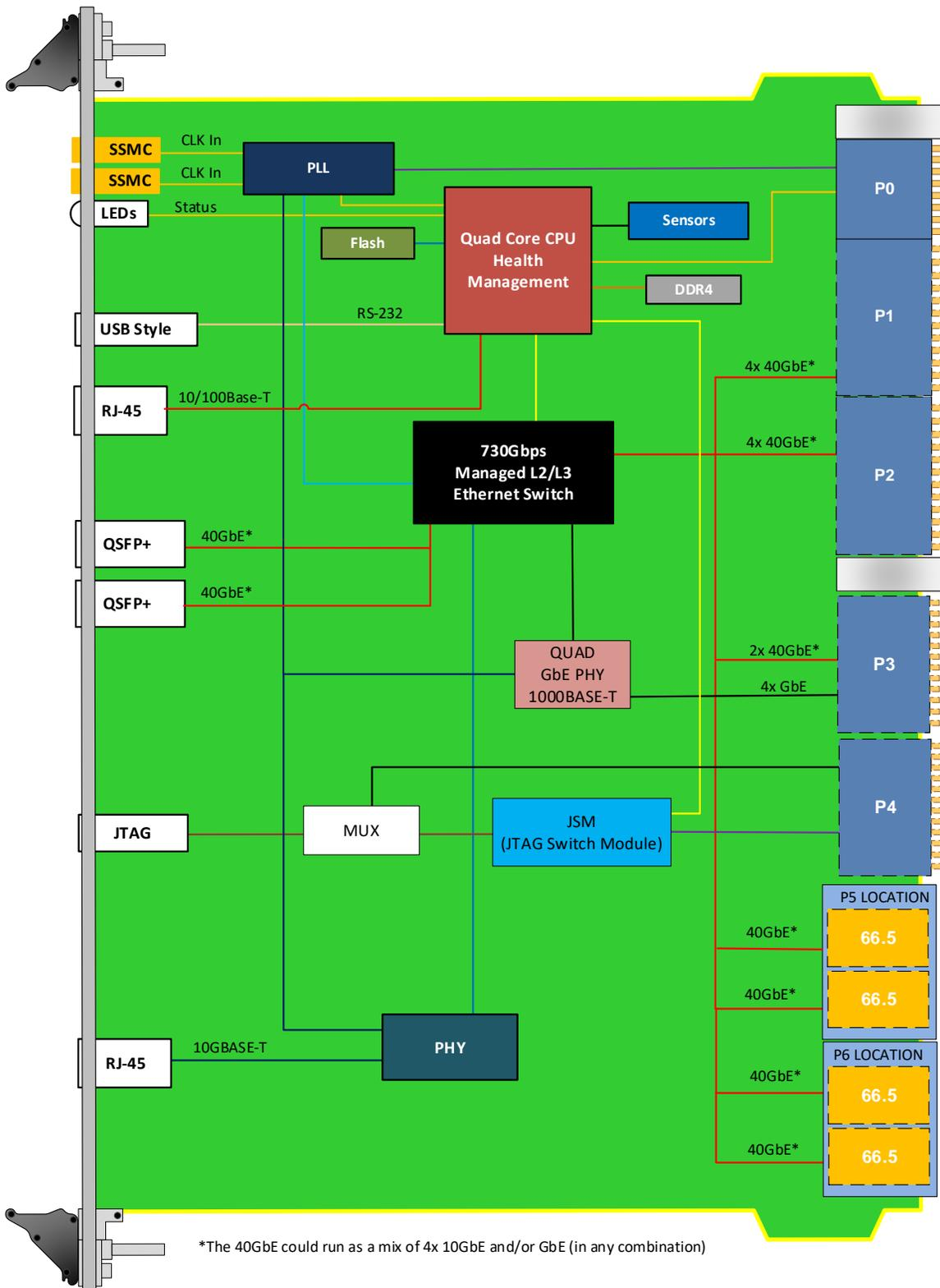
Figure 4: VPX011 Functional Block Diagram
