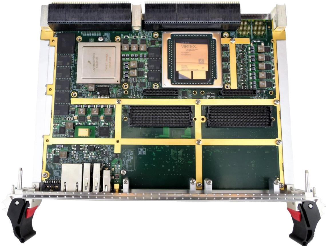
Figure 4: VPX554 Top View without Heatsink
