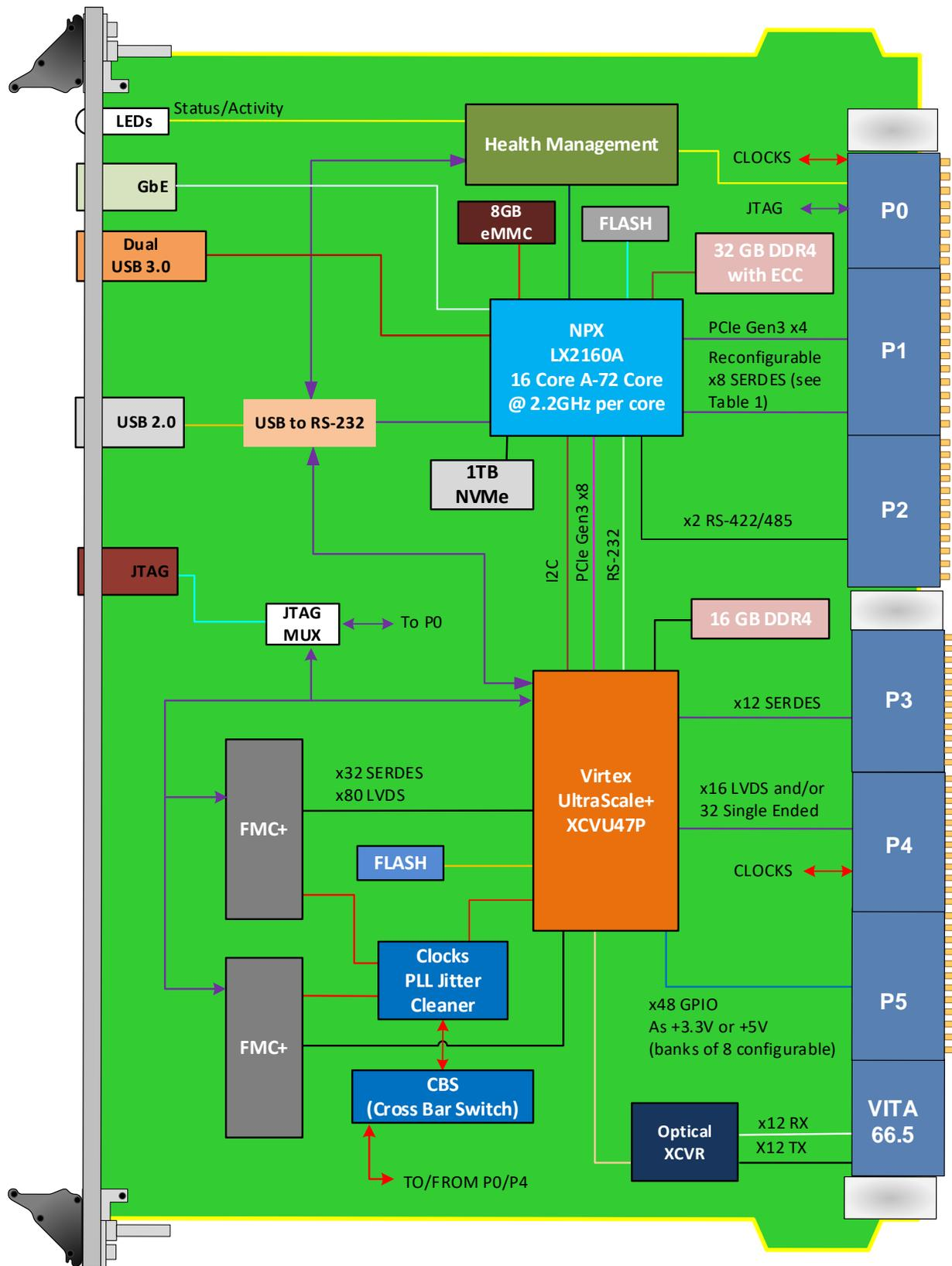
Figure 5: VPX554 Functional Block Diagram
