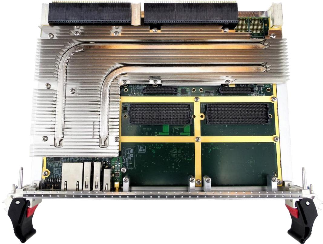
Figure 3: VPX554 Top View with Heatsink
