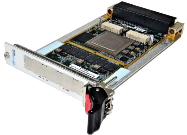
Figure 2: VPX705 without Heatsink
