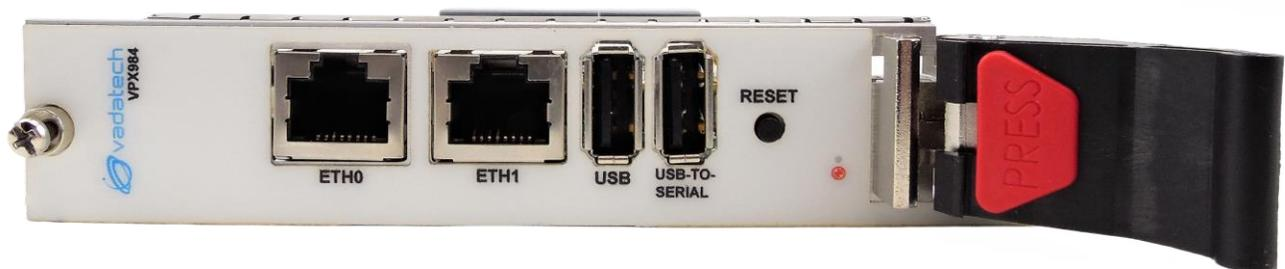
Figure 3: VPX984 Front Panel View
