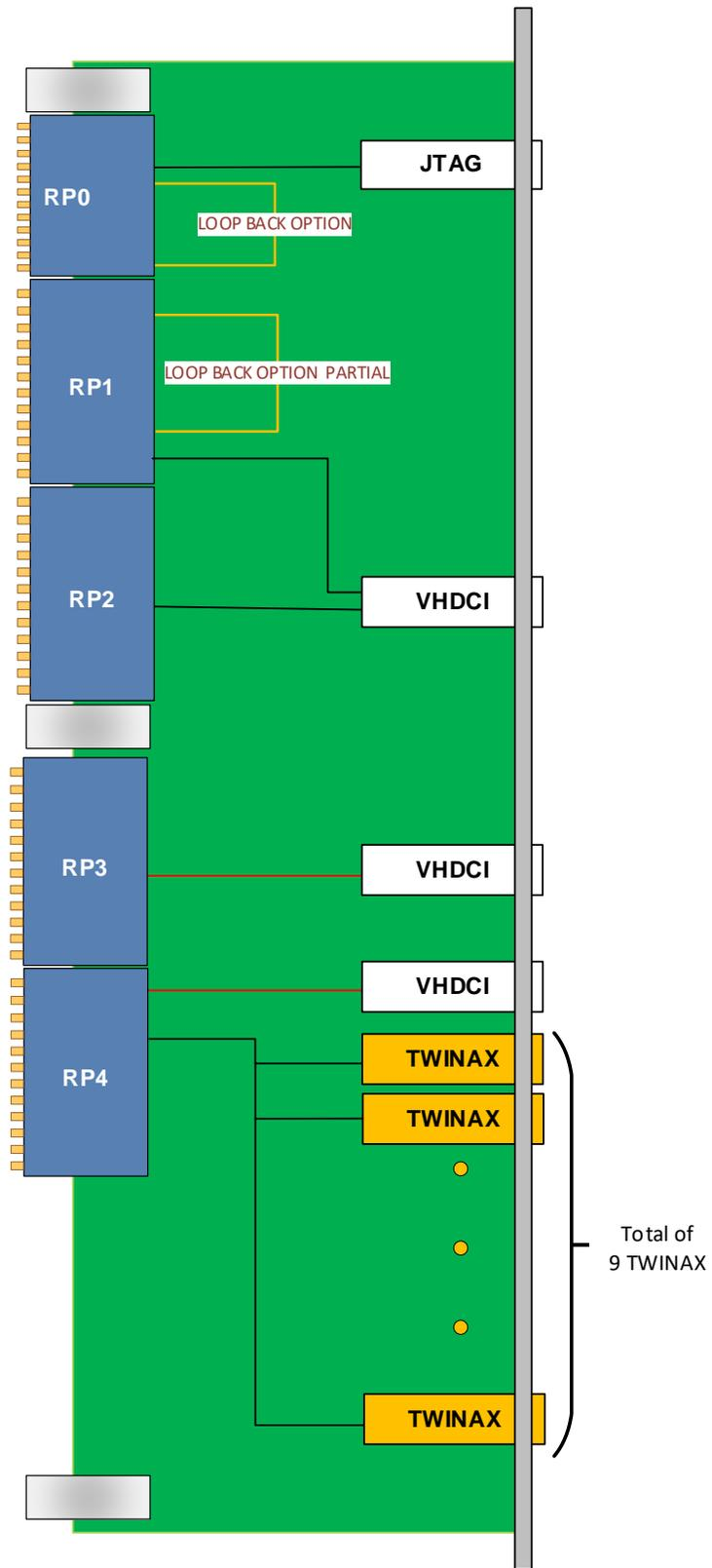
Figure 4: VRT556A Functional Block Diagram
