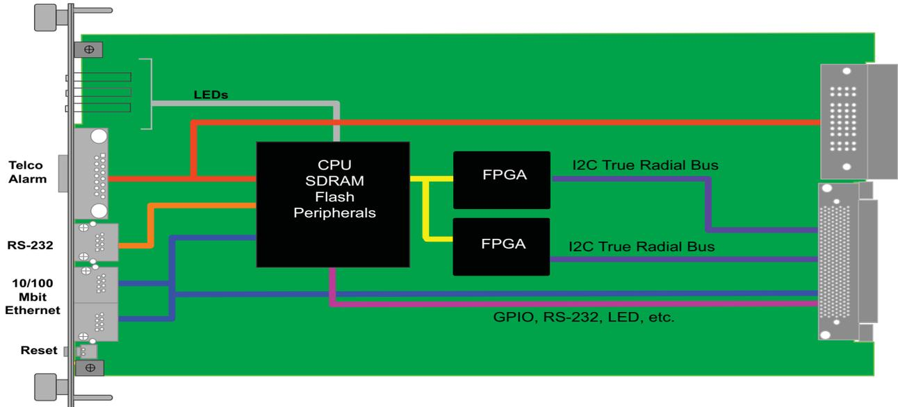
FIGURE 2. VT005 Functional Block Diagram
