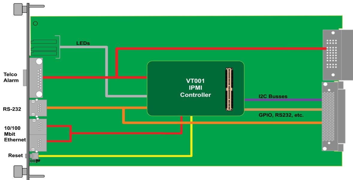
FIGURE 2. VT006 Functional Block Diagram and Front Panel
