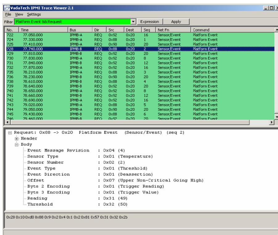
The screenshot shows the VadaTech IPMI Trace Viewer 2.1 interface. The main window displays a table of IPMI events with columns for No., Time, Bus, Dir, Src, Dest, Seq, Net Fn, and Command. A filter is set to 'Platform Event &&Request'. The selected event (No. 723) is expanded to show its body details:
