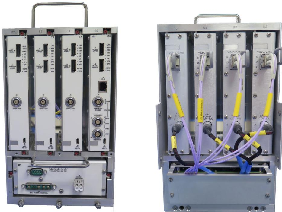
Figure 3: Conduction cool deployment example
