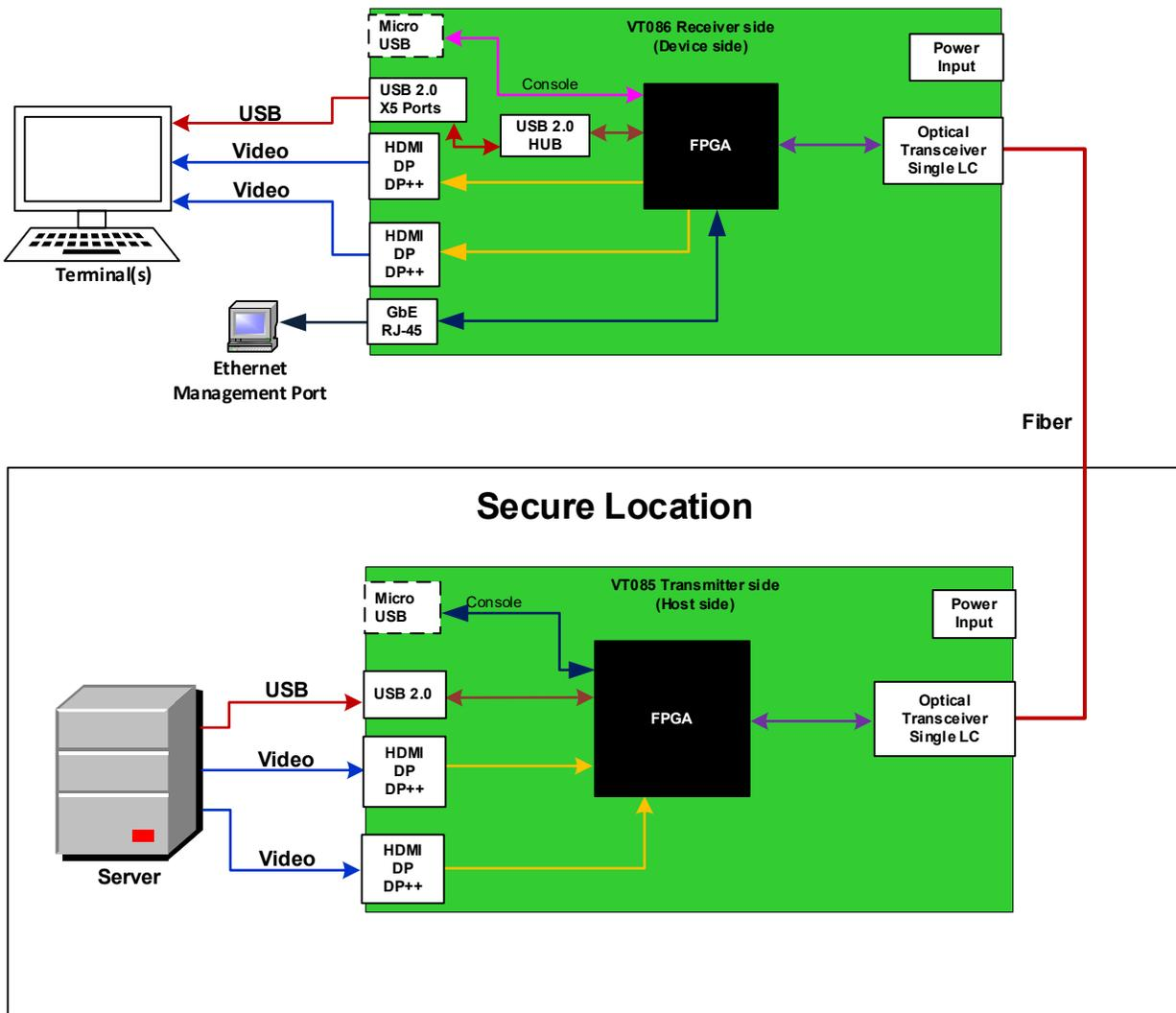
Figure 3: VT085/VT086 Connectivity Block Diagram
