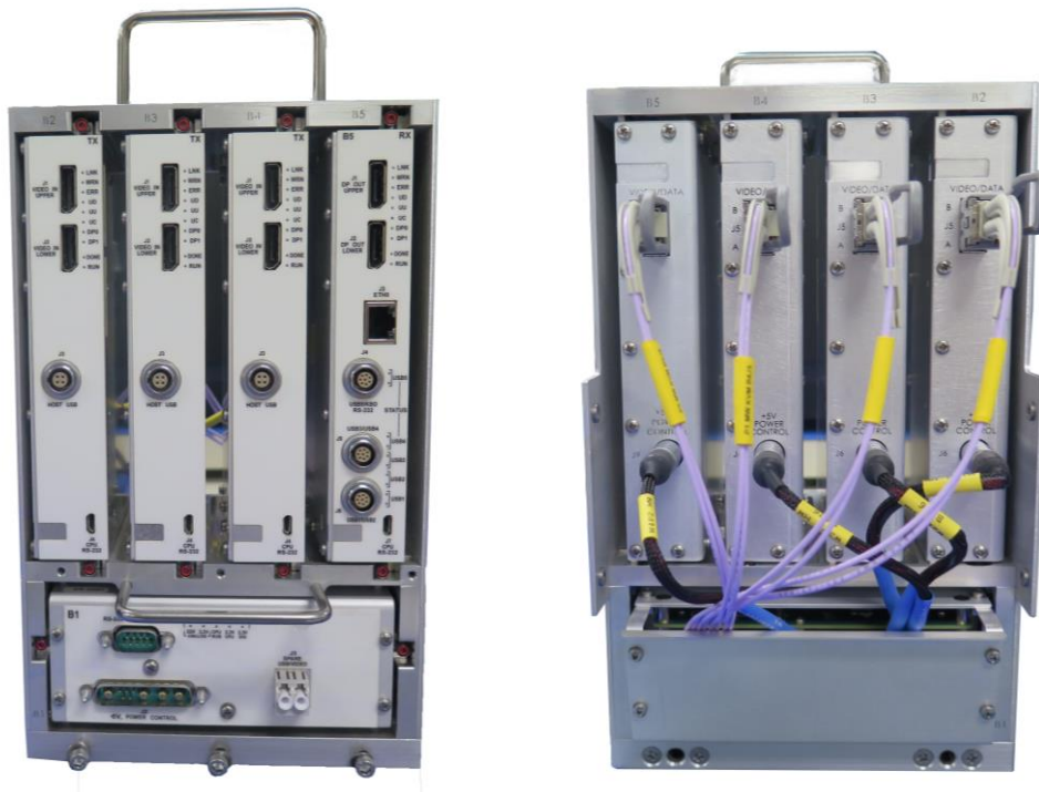
Figure 6: Conduction cool deployment example
