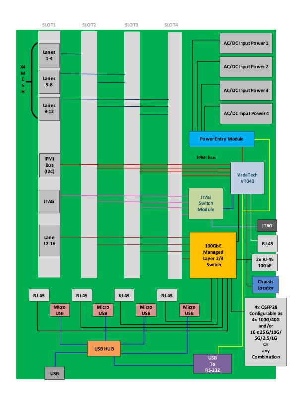
Figure 5: VT805 Backplane Connections (VadaTech can modify the motherboard for different topology)
