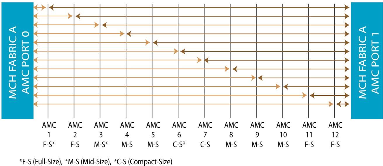
FIGURE 2. VT860 Topology for AMC Ports 0 and 1
