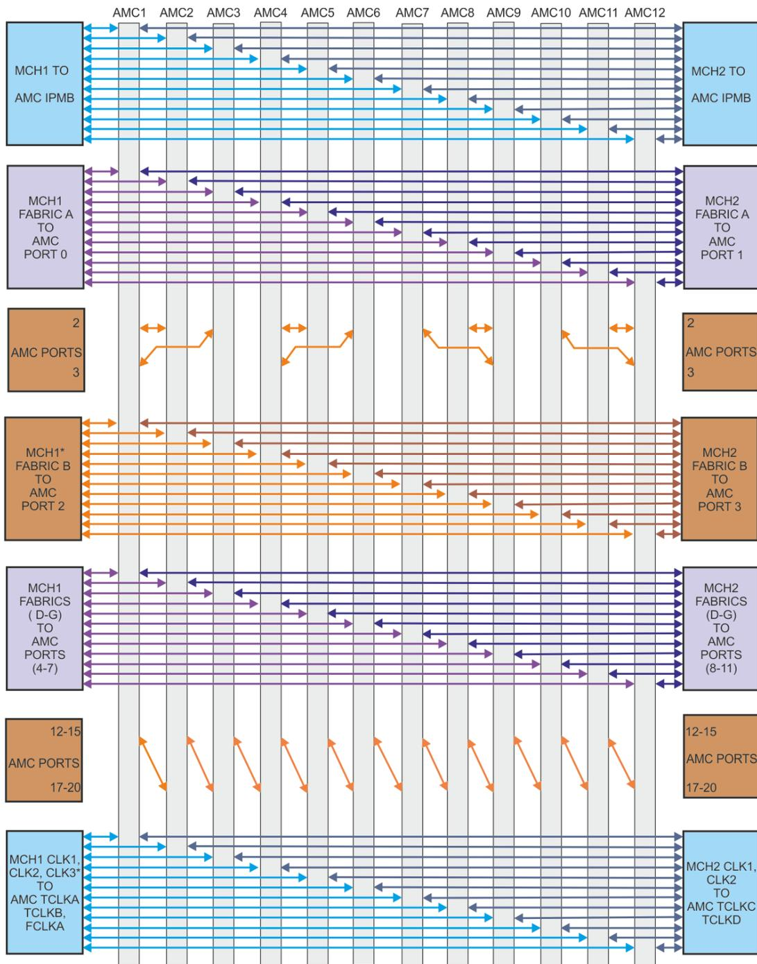
Figure 5: VT867 Backplane Connections
