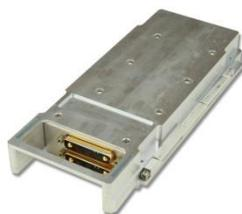
UTC011 Conduction Cooled Power Module
