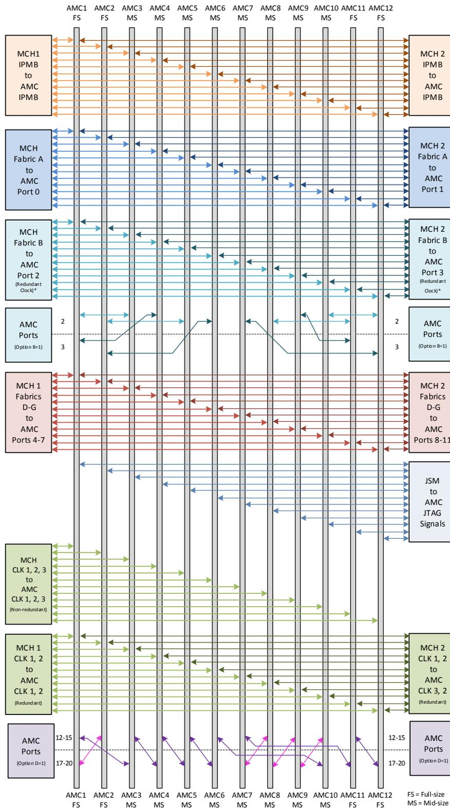
**Note:** When CLK3 is non-redundant, Fabric B will be partially provided only on ports 1 to 6. CLK3 is routed on Fabric B on ports 7 to 12.
