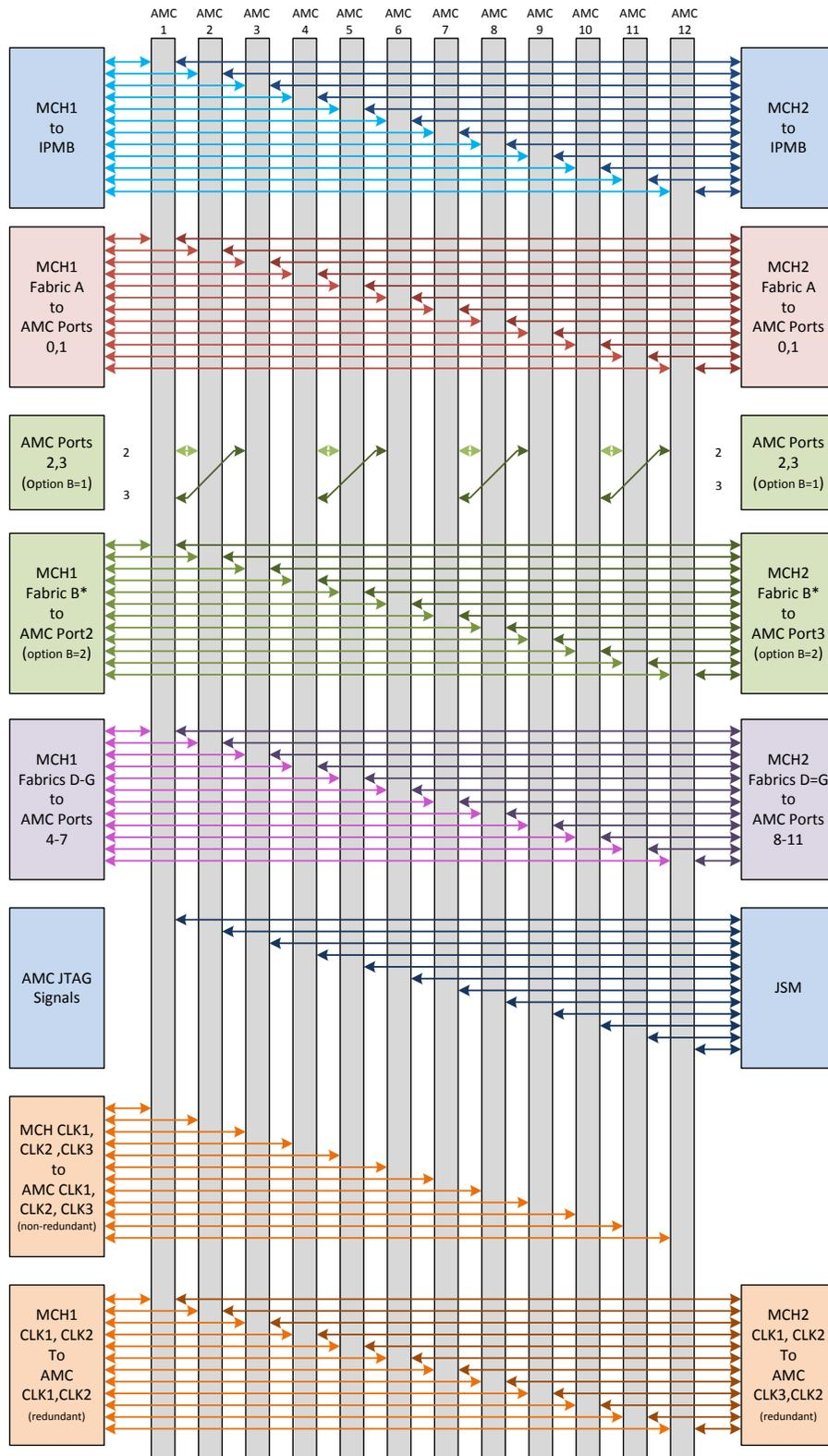
\*When CLK3 is non-redundant, Fabric B will be partially provided only on ports 1 to 6. CLK3 is routed on Fabric B on ports 7 to 12.
